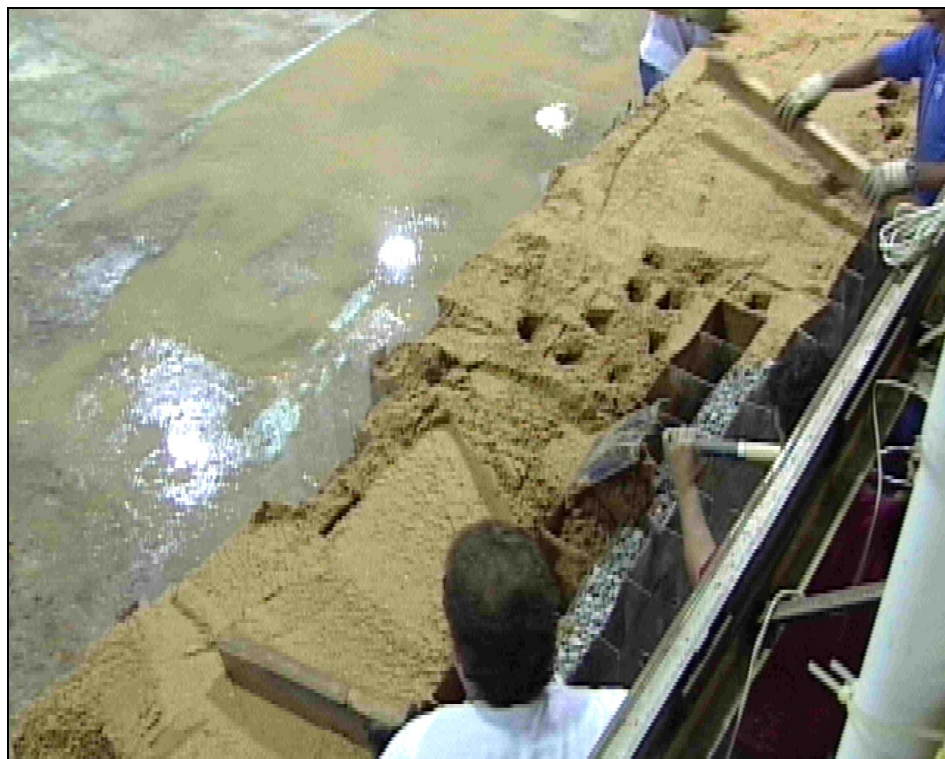
Figure 10. Compacting and screening sand in RDFW cells
