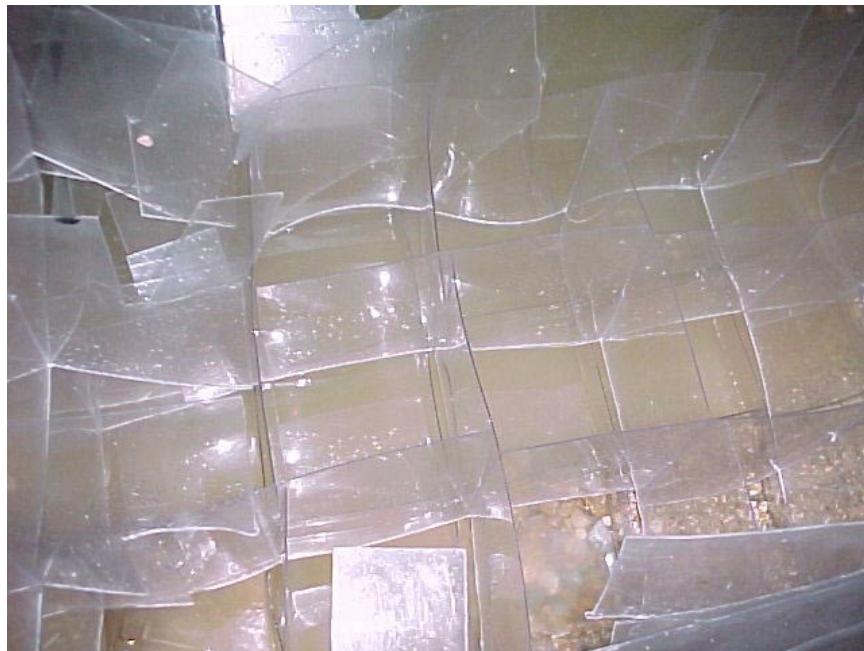
Figure 41. PETG plastic damage due to wave impacts
