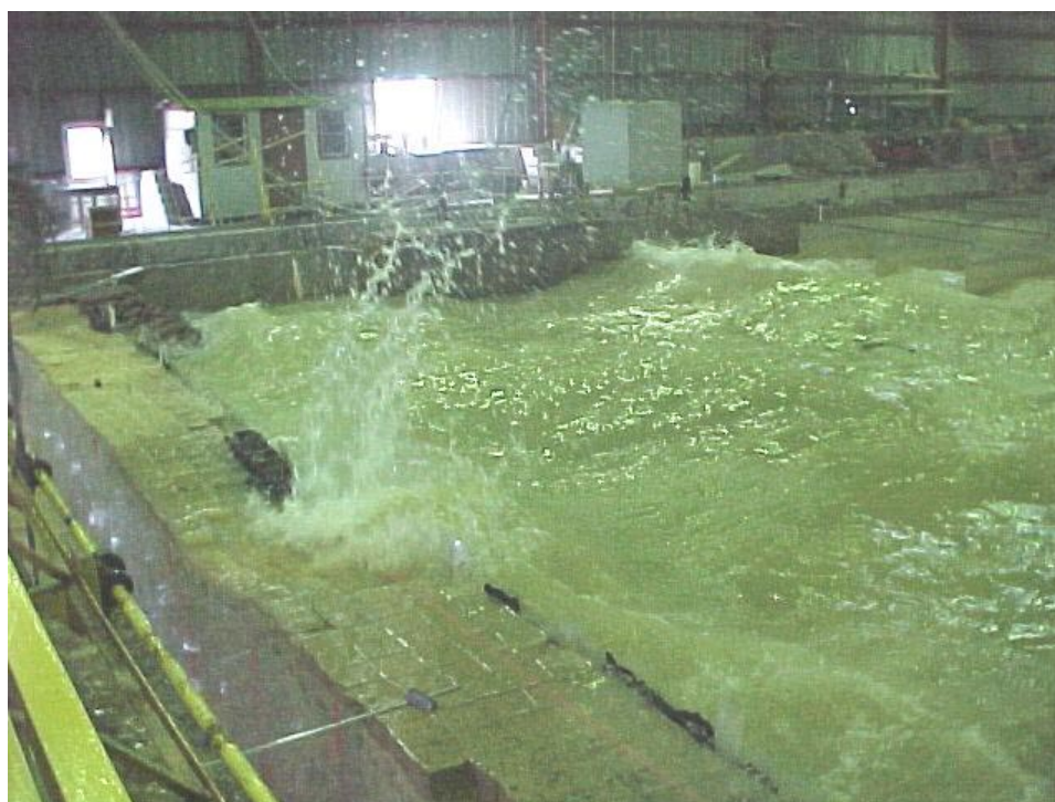
Figure 26. Overtopping at 45 percent gain, H = 1.49 ft, d = 2.0 ft
